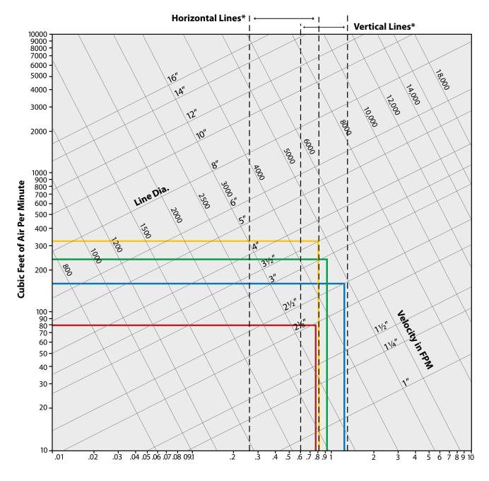
Friction loss in "Hg per 100 ft. of line with Inlet Air @ 68°F and 29.92" Hg.
