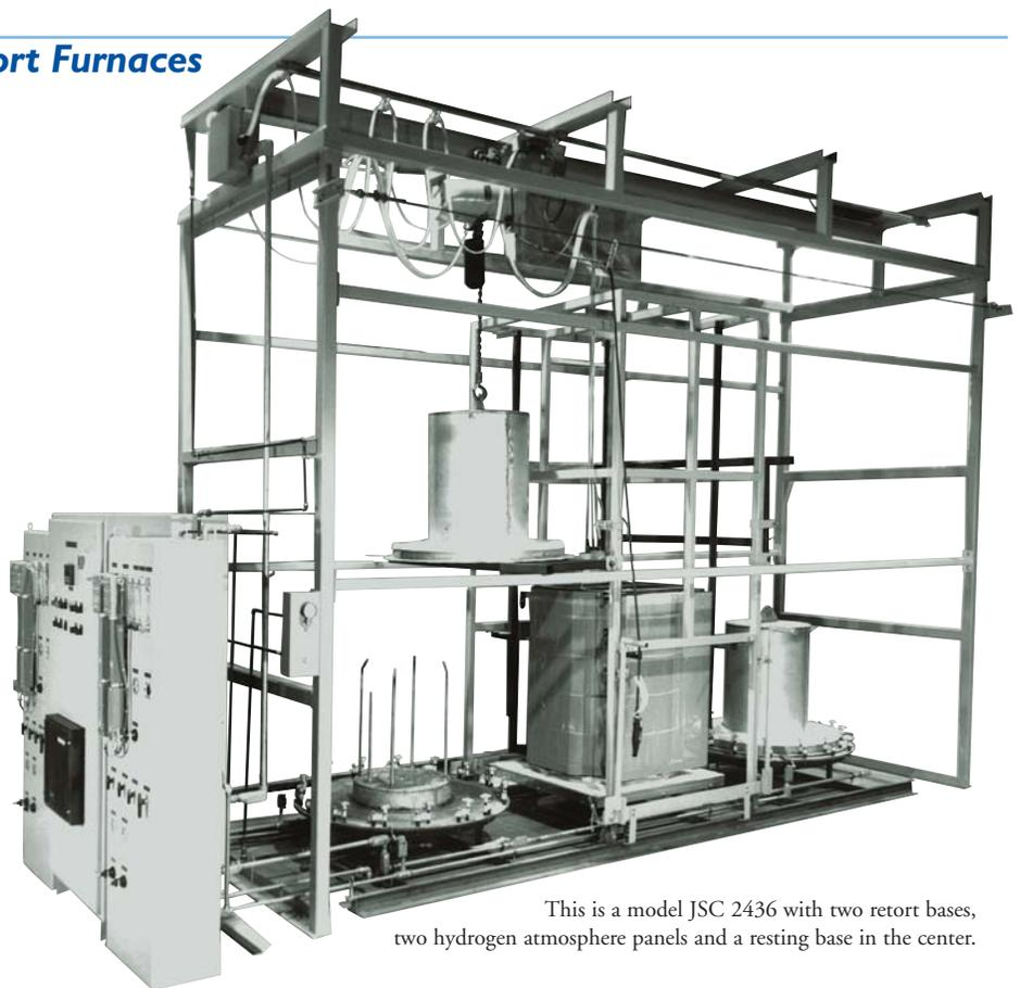
This is a model JSC 2436 with two retort bases, two hydrogen atmosphere panels and a resting base in the center.
