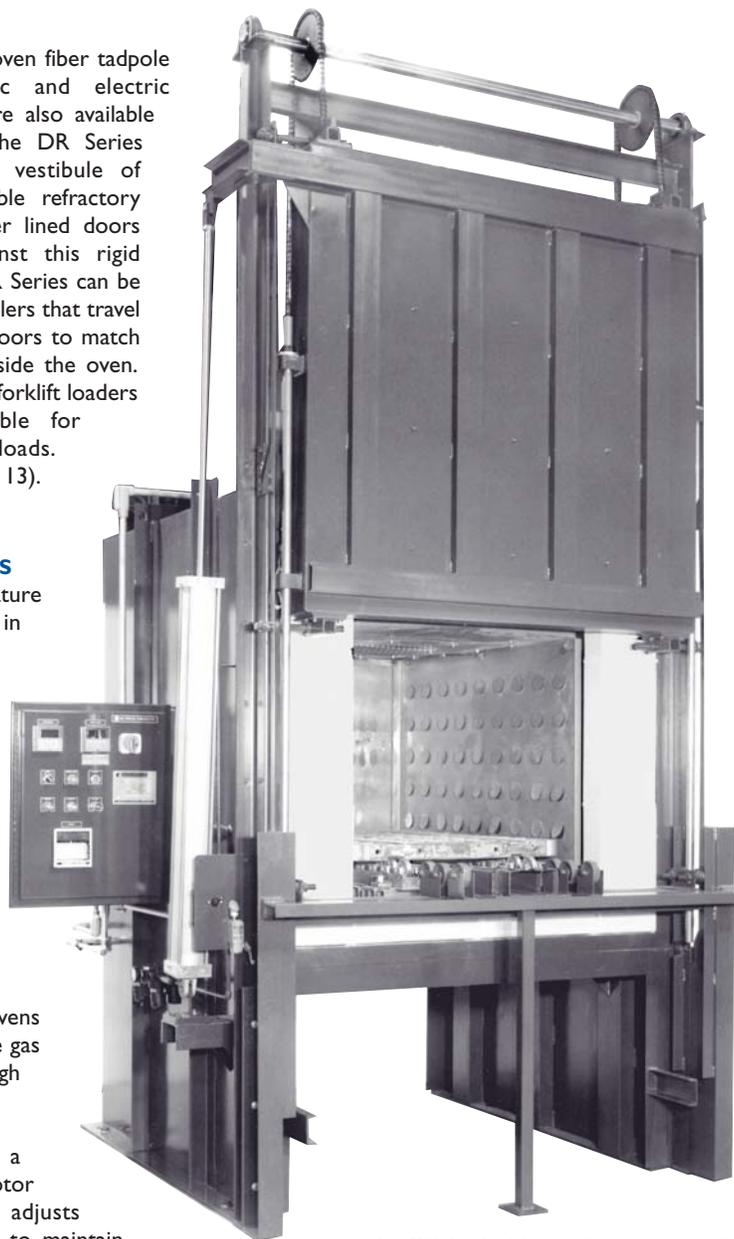
Above is a DR 3648 with a vertical door and roller hearth system. You can see the recirculation muffle inside with adjustable air louvers. These allow you to adjust the pattern of high velocity air inside the oven to achieve maximum temperature uniformity.
