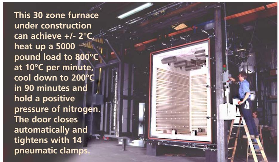
This 30 zone furnace under construction can achieve +/- 2°C, heat up a 5000 pound load to 800°C at 10°C per minute, cool down to 200°C in 90 minutes and hold a positive pressure of nitrogen. The door closes automatically and tightens with 14 pneumatic clamps.
