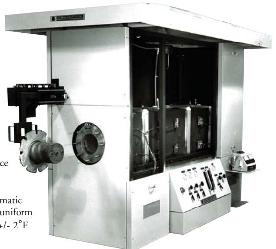
This hydrogen tube furnace is used for processing monochromatic glass. It is uniform to within +/- 2°F.
