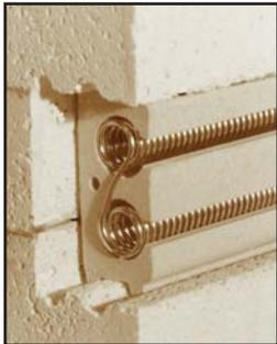
element and excellent radiating characteristics. The smooth surface of the holder prevents premature failure of the element as it expands and contracts. These holders, coupled with a unique all ceramic
