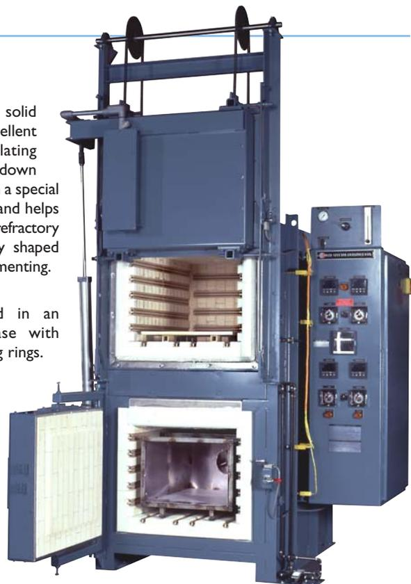
This QD 236 features a pneumatic vertical door with a foot switch, atmosphere sealed case on top, NEMA 12 control panel and strip chart recorder.
