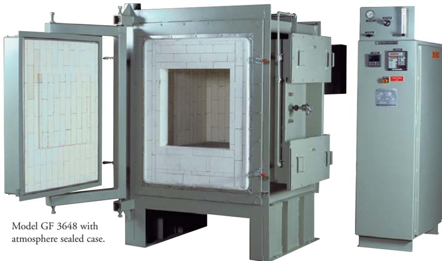
Model GF 3648 with atmosphere sealed case.
