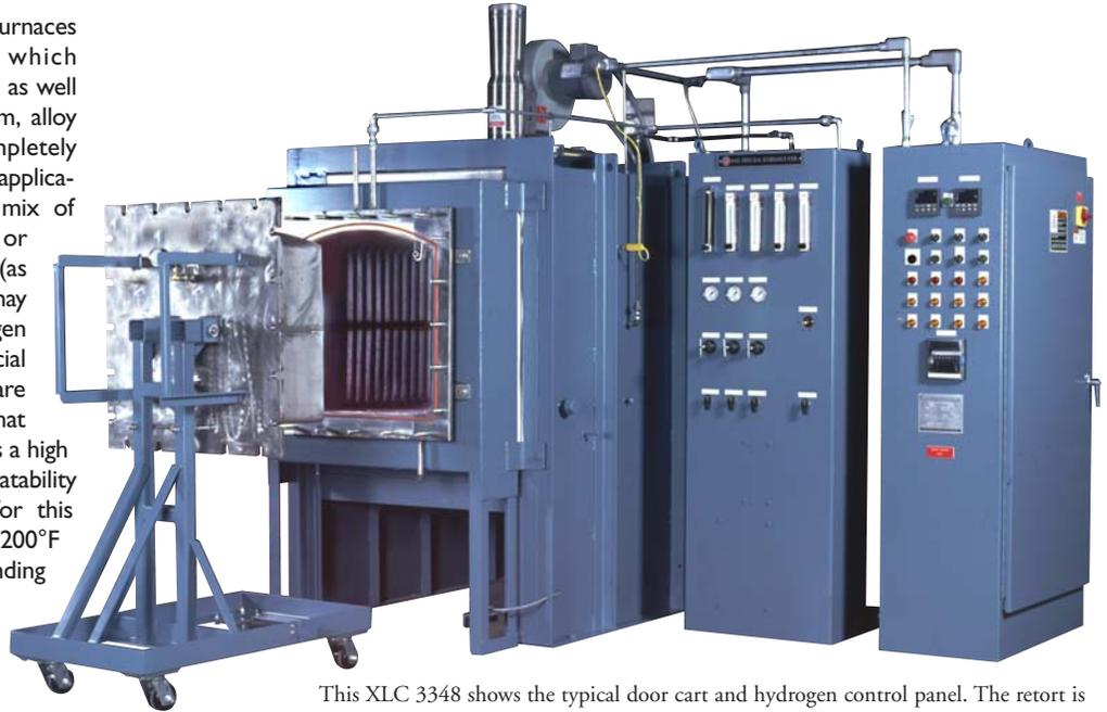
This XLC 3348 shows the typical door cart and hydrogen control panel. The retort is "D" shaped corrugated Inconel for the highest possible strength. A venturi cooler is also shown.
