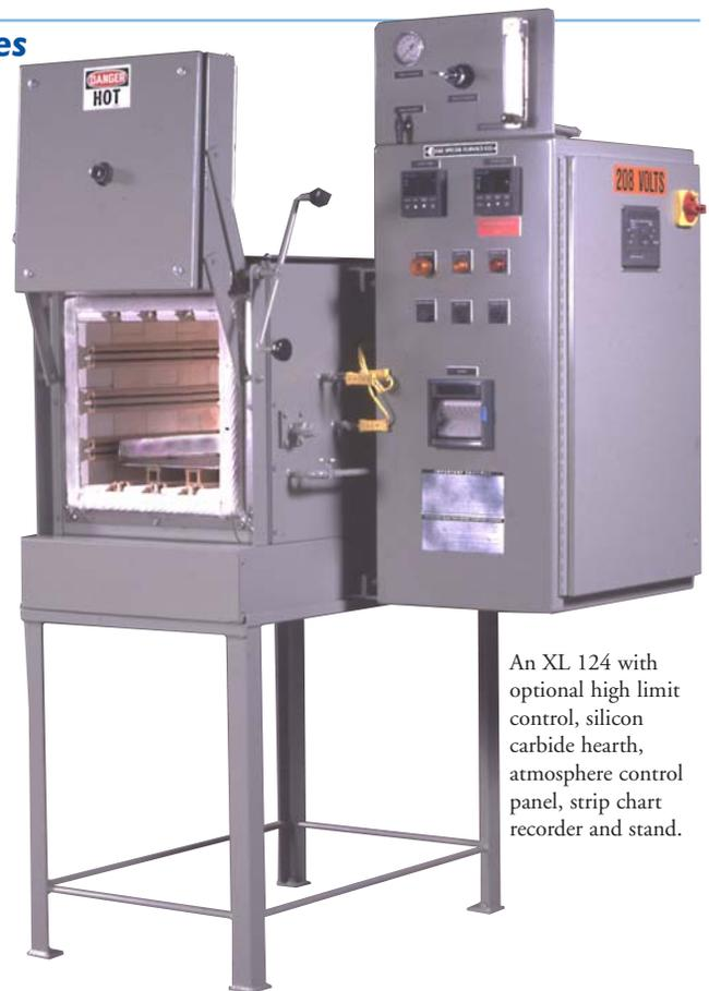
An XL 124 with optional high limit control, silicon carbide hearth, atmosphere control panel, strip chart recorder and stand.
