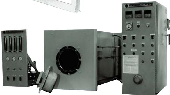
This is a TBU 1424 with a hydrogen retort and H2 Atmosphere panel.
