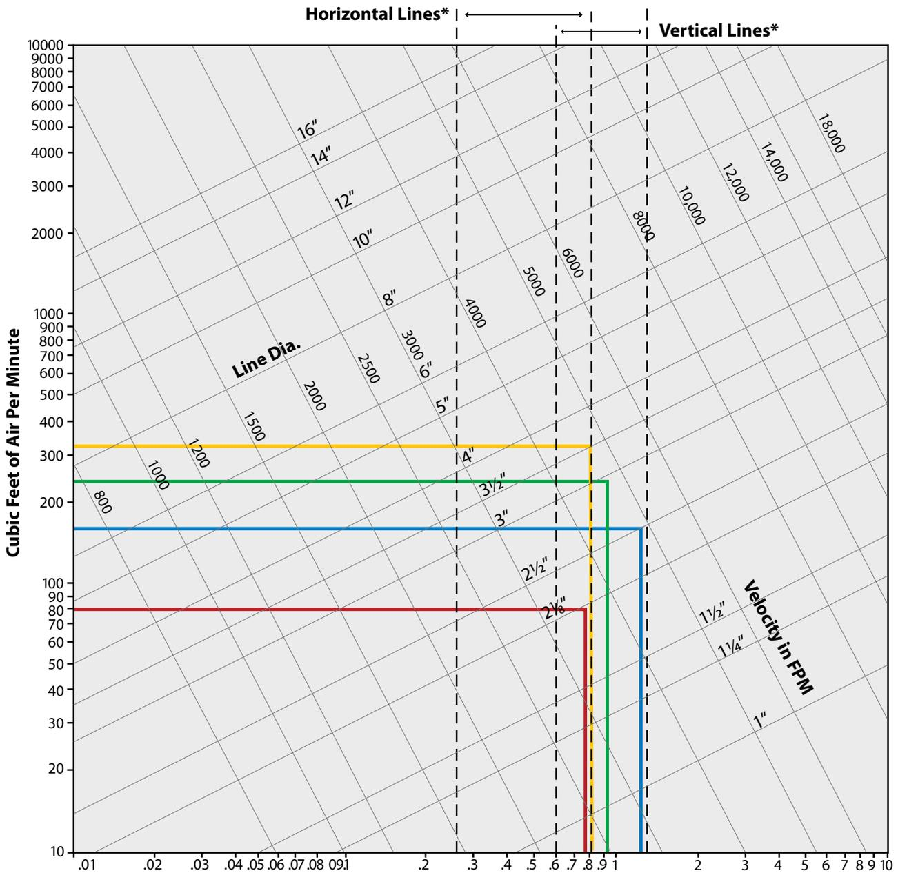
Friction loss in "Hg per 100 ft. of line with Inlet Air @ 68°F and 29.92" Hg.
